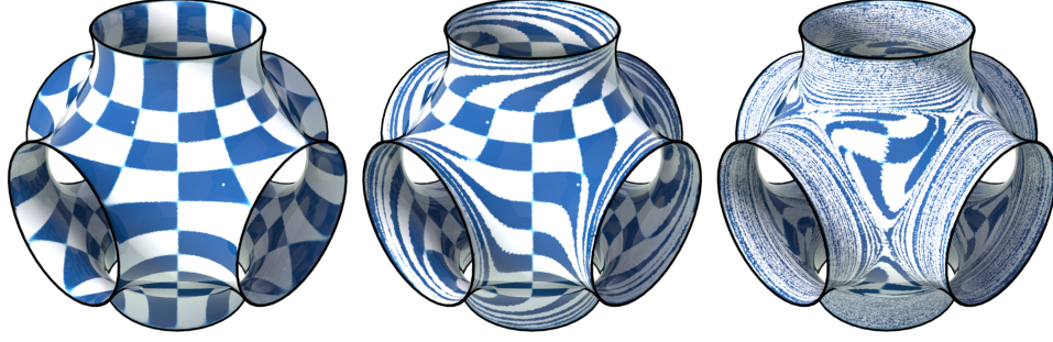
Figure 2.5. On the Schwarz P surface, an initially stationary fluid ( w = 0 , c = \mathbf{0} ) is set into motion by a rotating boundary with prescribed velocity \bar{u}_\partial = 2 . The no-slip condition (2.52) is enforced using Algorithm 2 with time step \Delta t = 0.01 . Each boundary circle has radius 0.4, and the viscosity is set to \nu = 0.01 .
